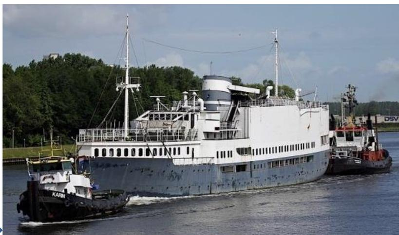
*HSS Discovery* (ex-*Stena Discovery*). IMO 9107590. High-speed ship. 122 m long. Venezuelan flag. Unknown classification society. Built in 1997 in Rauma (Finland) by Finnyards Oy. The fast ship *Stena Discovery*, after having assured the connection in the North Sea between Hoek van Holland and Harwich for Stena Line, was decommissioned in 2007 due to high bunker costs.
